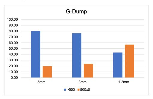
Figure 7: Size comparisons of G-dump crushed at 5mm, 3mm and 1.2mm
