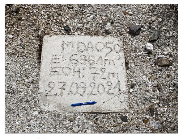
Figure 10-4: Concrete Plinth Over Collar MDA050
