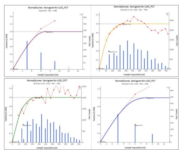
Figure 14-8: Semivariograms for the K-Dump for Li<sub>2</sub>O %
