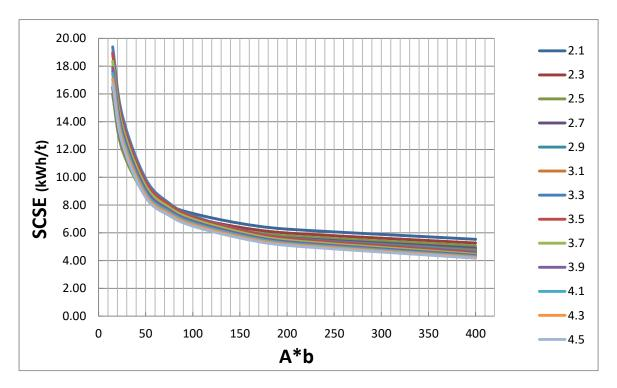
App Figure 3 – The relationship between A\*b and specific energy at varying SG for the "Standard" circuit.
