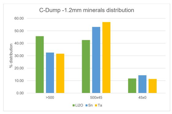
Figure 12: Valuable minerals distribution of C-dump crushed down to 1.2mm
