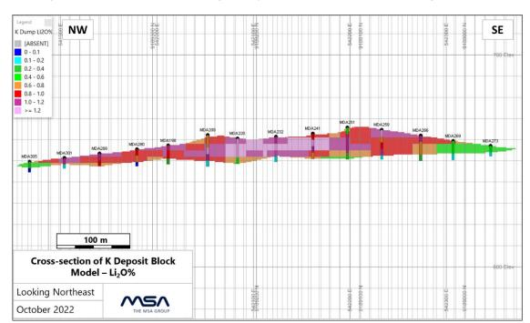
Figure 14-12: Cross-Section Through K Deposit Coloured on Li<sub>2</sub>O % (Looking Northeast)
