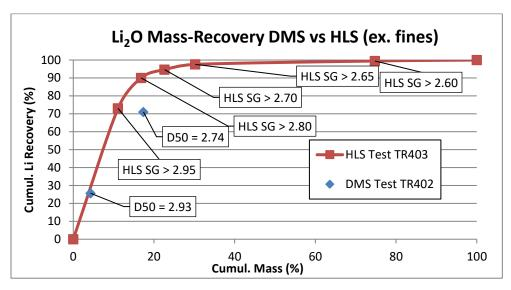
Figure 4: Mass-Recovery Comparison for DMS and HLS, K-G Blend Sample
