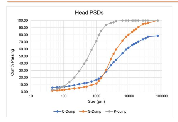
Figure 3: Particle size distribution of "as received" sample from C, G and K dumps
