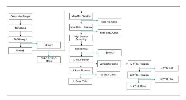
Figure 12: Flotation Test Flowsheet – Test F7
