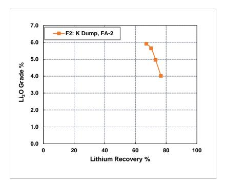
Figure 8: Li<sub>2</sub>O Grade vs. Lithium Recovery - Test F2 on the K-dump DMS Fines Fractions
