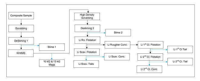
Figure 13: Flotation Test Flowsheet – Test F8
