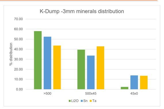
Figure 17: Valuable minerals distribution of K-dump crushed down to 3mm
