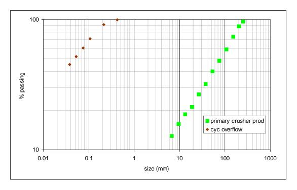
App Figure 9 – Example of a Typical Primary Crusher (Open and Circuit) Product Distribution Compared with a Typical Ball Mill Cyclone Overflow Distribution
