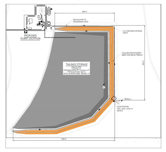
Figure 18-5: Tailings Storage Facility Layout
