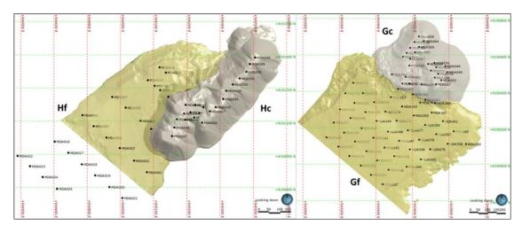
Figure 10-2: Manono Lithium Tailings Project Drillhole Collars for Hc, Hf, Gc and Gf Deposits
