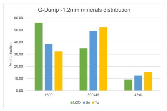
Figure 15: Valuable minerals distribution of G-dump crushed down to 1.2mm
