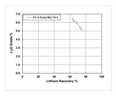
Figure 9: Li<sub>2</sub>O Grade vs. Lithium Recovery - Test F3 on the G-dump DMS Middlings
