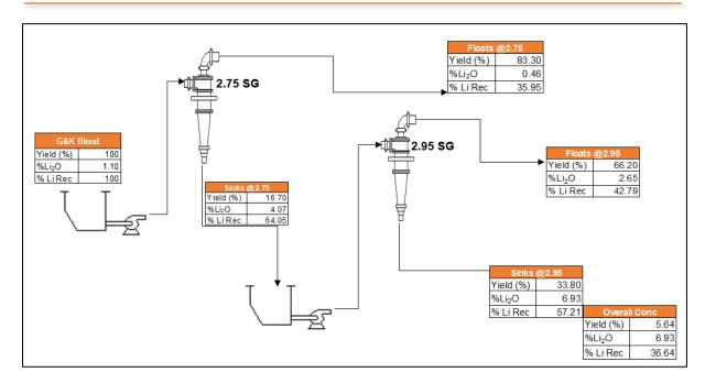
Figure 19: Overview of DMS testwork on the blend (G&K)
