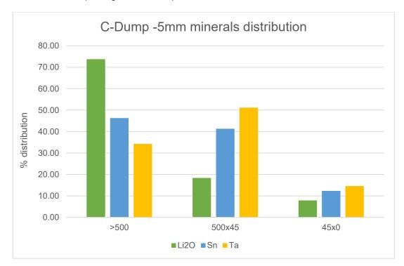
Figure 10: Valuable minerals distribution of C-dump crushed down to 5mm
