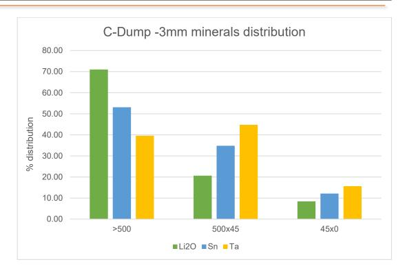
Figure 11: Valuable minerals distribution of C-dump crushed down to 3mm
