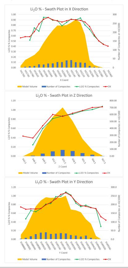
The block model was examined visually to ensure that the drillhole grades were locally well represented by the block model and it was found that the model validated reasonably well, with acceptable degrees of smoothing observed for all attributes. Examples of visual validation of the models for the K deposit in plan view and section are shown in Figure 14-11 and Figure 14-12 respectively.
