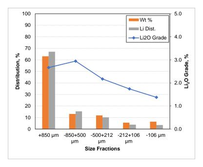
Figure 10: Size Fractional Analysis Results - G-dump DMS Middlings (100% passing 6 Mesh (3.35 mm)
