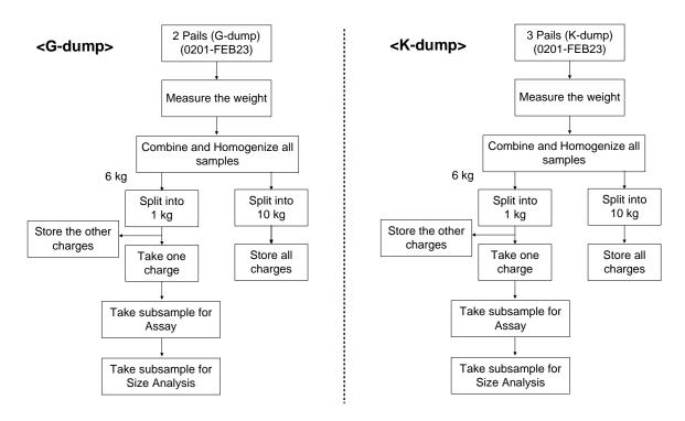
Figure 2: Sample Preparation Flowsheet for the DMS Fines Fractions
