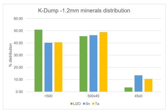
Figure 18: Valuable minerals distribution of K-dump crushed down to 1.2mm
