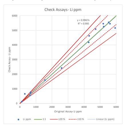
Figure 12-2: Scattergram for Lithium – Check vs. Original Samples
