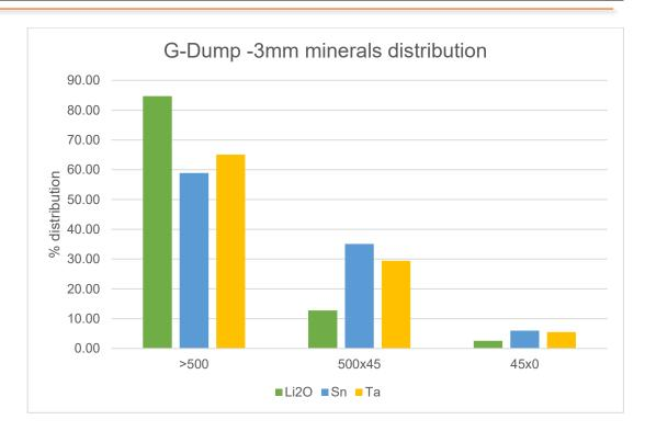
Figure 14: Valuable minerals distribution of G-dump crushed down to 3mm
