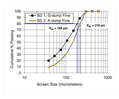
Figure 5: Particle Size Distribution on the SG 1 and the SG 2
