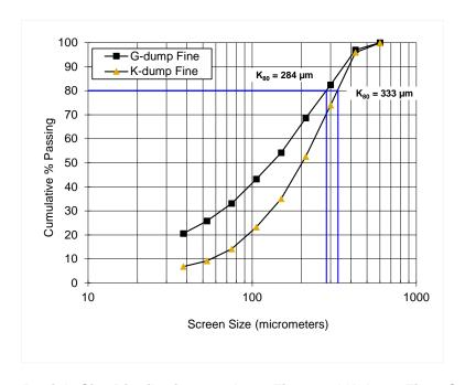
Figure 4: Particle Size Distribution – G-dump Fines and K-dump Fines Samples
