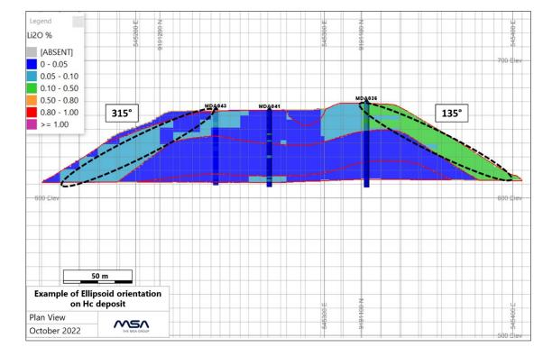
Figure 14-9: Example of Search Ellipsoid Orientation Used for the Hc Deposit
