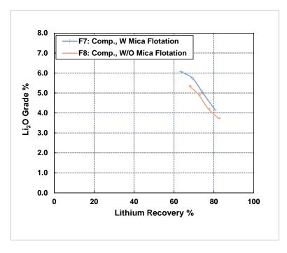
Figure 14: Li<sub>2</sub>O Grade vs. Lithium Recovery – Tests F7 and F8 on the Composite Samples with/without Mica Flotation
