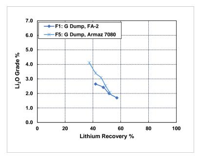
Figure 7: Lithium Flotation Test Results (F1 and F5)
