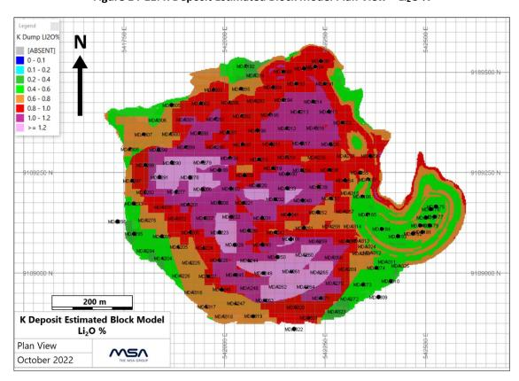
Figure 14-11: K Deposit Estimated Block Model Plan View - Li<sub>2</sub>O %
