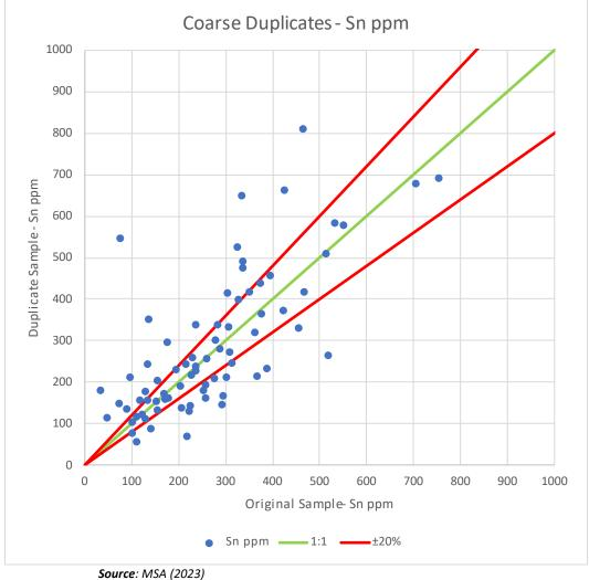
Figure 11-13: Precision of Tin in 78 Coarse Duplicate Pairs
