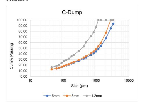
Figure 4:Particle size distribution of C-dump crushed at 5mm, 3mm and 1.2mm Crushing at 5 and 3mm generated approximately 20% of fine (<500 $\mu$ m) material, whereas crushing at 1.2mm generated up to 60% fine material (<500 $\mu$ m) as seen in Figure 5.
