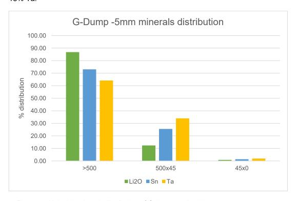
Figure 13: Valuable minerals distribution of G-dump crushed down to 5mm
