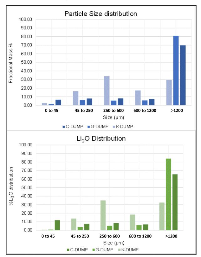
A summary of the HLS results is available in Table 13-5. The HLS test produced spodumene concentrate grades of  $6.5\%~\text{Li}_2\text{O}$  at overall recoveries across the size range of 47% and 63% for G-dump and K-dump respectively. The testwork did not produce a SC6 product from the C-dump, this requiring further investigation. These results are for all the dump material with a PSD smaller than 5 mm.
