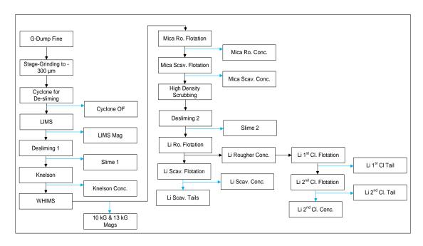
Figure 6: Flotation Test Flowsheet – Tests F1 and F5
