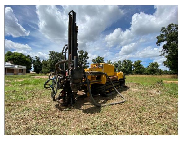
Figure 11-3: Track Mounted Aircore Rig with Mounted Cyclone
