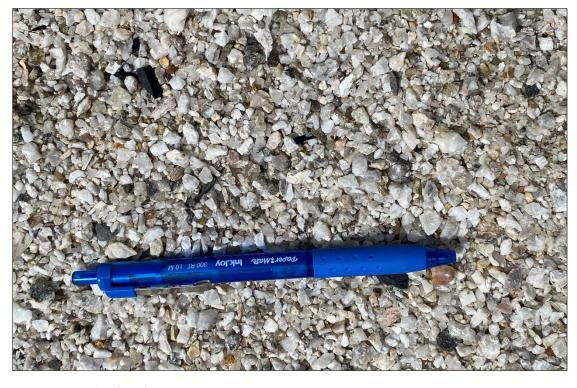
Figure 7-3: Manono Lithium Tailings Project Coarse Tailings Material
