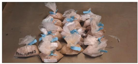
Figure 12-1: Sealed Check Samples from Manono at COAL
