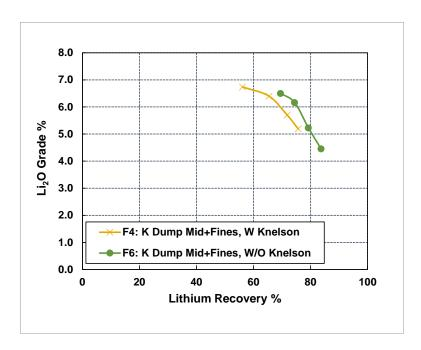
Figure 11: Li₂O Grade vs. Lithium Recovery – Tests F4 and F6 on the K-dump DMS Middlings with and without Knelson Separator
