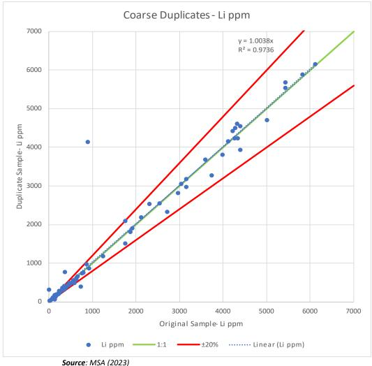
Figure 11-12: Precision of Lithium in 108 Coarse Duplicate Pairs
