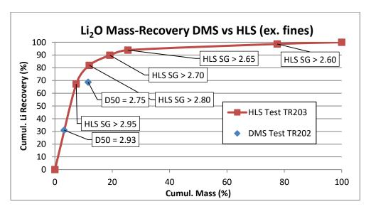
Figure 3: Mass-Recovery Comparison for DMS and HLS, G-Dump Sample
