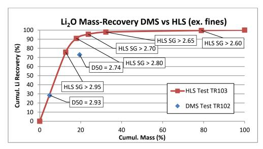
Figure 2: Mass-Recovery Comparison for DMS and HLS, K-Dump Sample
