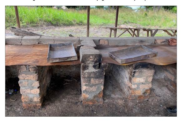
Figure 11-4: Wood Fire Ovens and Drying Pans Used to Dry Samples
