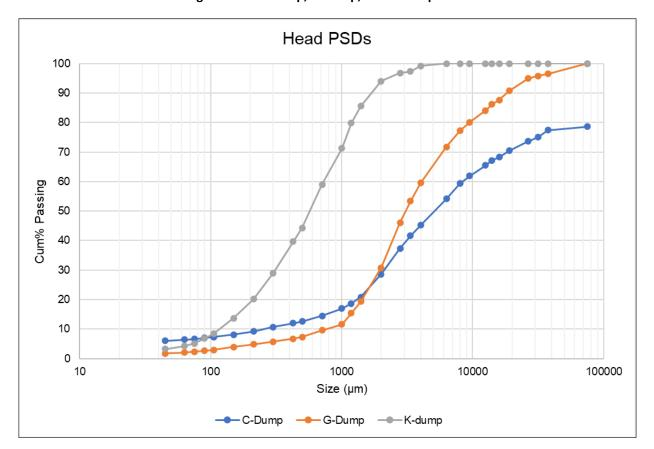
Figure 13-4: K-dump, G-dump, and C-dump PSDs
