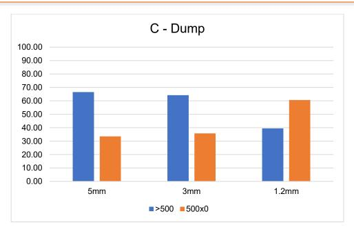
Figure 5: Size comparisons of C-dump crushed at 5mm, 3mm and 1.2mm
