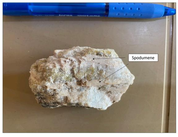
Figure 7-7: Pegmatite Sample from Manono Illustrating Prismatic Cleavage
