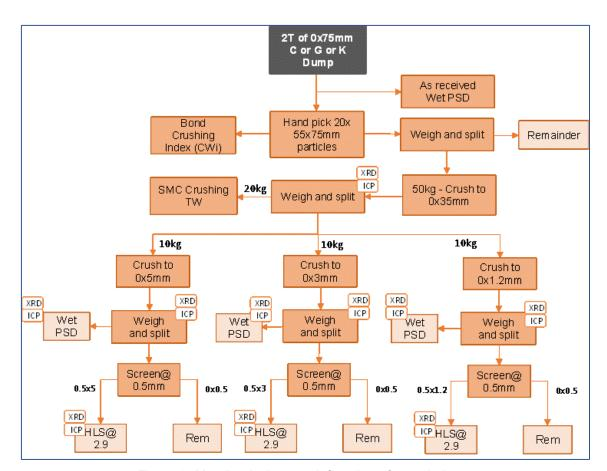
Figure 2: Metallurgical testwork flowsheet for each dump
