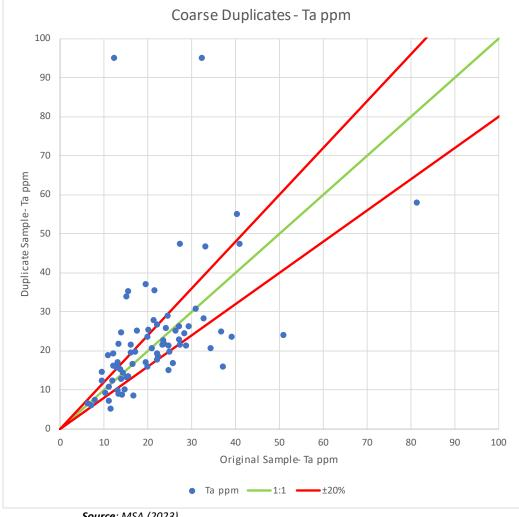
Figure 11-14: Precision of Tantalum in 78 Coarse Duplicate Pairs
