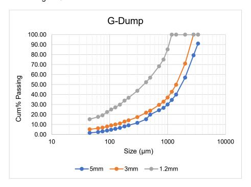
Figure 6:Particle size distribution of G-dump crushed at 5mm, 3mm and 1.2mm
