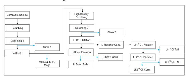
Figure 13-7: SGS Flotation Test Flowsheet
