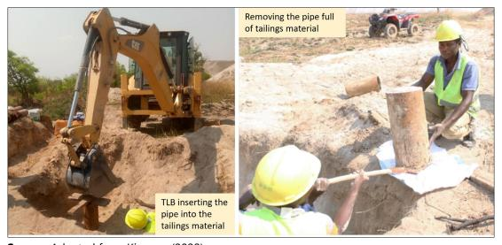
Figure 11-18: Bulk Density Sampling
