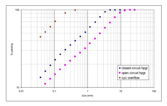
App Figure 10 – Examples of Open and Closed Circuit HPGR Distributions Compared with a Typical Ball Mill Cyclone Overflow Distribution
