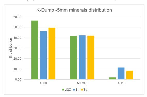
Figure 16: Valuable minerals distribution of K-dump crushed down to 5mm
